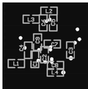
Figure 25. Bottom Layer Silkscreen
